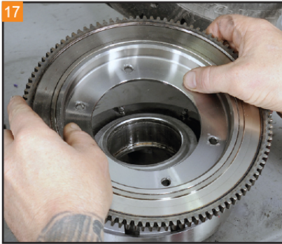
17 Remove the starter ring gear from the stock clutch basket.
