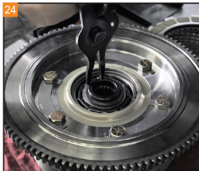
24 Install the retaining ring into the clutch hub from the transmission side.
