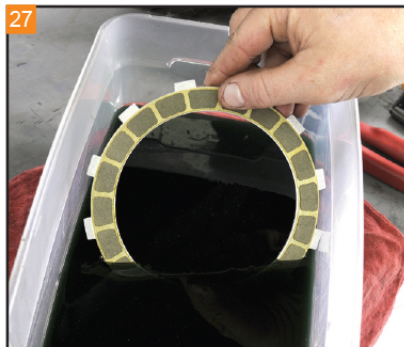
27 Allow the clutch plates to soak for 10 minutes prior to installation.
