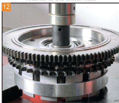
12 Use a hydraulic press to press the clutch hub from the bearing.
