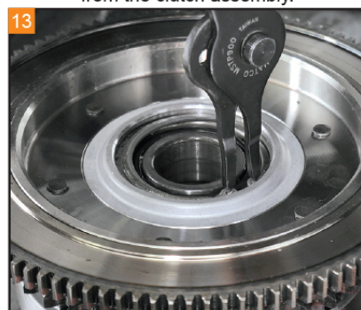
13 Remove the bearing-retaining ring from the clutch basket.
