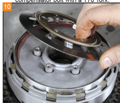
10 Remove the retainer, spring, pressure plate, and clutch plates from the clutch assembly.
