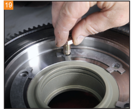
19 Position the ring gear over the Barnett clutch basket. Install the included bolts and locking tabs.
