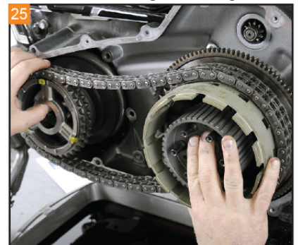
25 Install the clutch assembly, primary chain, and compensating sprocket. Ensure the primary chain is running the same direction as before.
