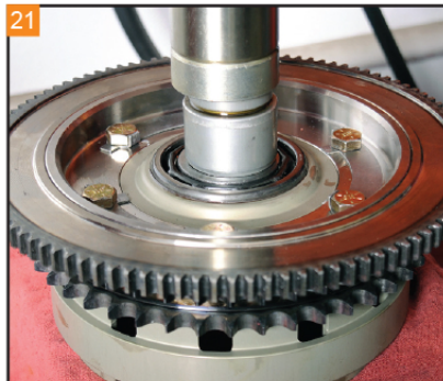
21 Verify the stock bearing spins freely. Press in the bearing into the Barnett Clutch Basket from the transmission side.
