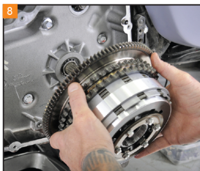
8 After removing the compensating sprocket and primary chain, remove the clutch assembly from the mainshaft.
