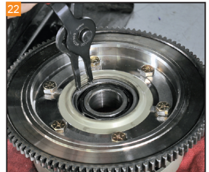
22 Install the retaining ring into the appropriate groove for your application, flat side facing the bearing.
