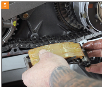
5 Use a 1/2" socket to remove the two bolts holding the primary chain adjuster. Keep a hand on the adjuster while removing it, it is spring loaded.
