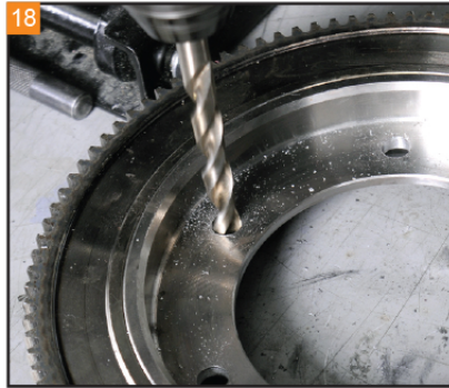
18 Open the holes in the ring gear with a 3/8" bit.
