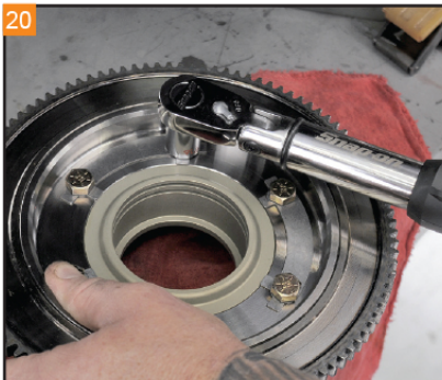
20 Tighten the bolts in a criss-cross pattern. Final torque of 25 foot/lbs. Bend one locking tab per bolt onto a flat of each bolt.
