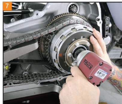
7 Install the primary locking tool. Use an impact wrench to remove the mainshaft nut. This nut is left-hand thread. Reverse the primary locking tool. Remove the compensator bolt with a T70 Torx.
